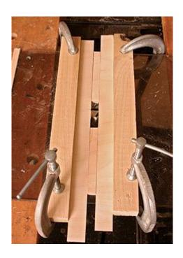
**Set up the jig.** Cut the center strip in two, raise the router bit to a height of 1/4 in., and place all of the spacers on the router table as shown. Turn the bit so it touches the outside spacers. Then clamp two thicker, outer guides in place (see above) to create a track for the drawer side. Now you can remove the spacers.
