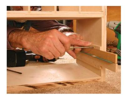
**Install the drawer runners.** After installing the gallery, install the drawer runners using the same shim stock and the two outside spacers from the router-table setup. To install the lowest pair of runners, stack a single shim, one of the outside spacers, and a drawer runner inside the cabinet, and screw the runner into place. To install each subsequent runner (see above), stack one outer spacer, a shim, and another outer spacer onto the last
