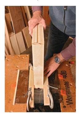
**Rout the drawer groove.** Use the track to rout a centered, 1/4-in.-deep groove in the side of each drawer. Mark a stopping point on the router table so the groove ends just before reaching the finger joints at the front of the drawer box.
